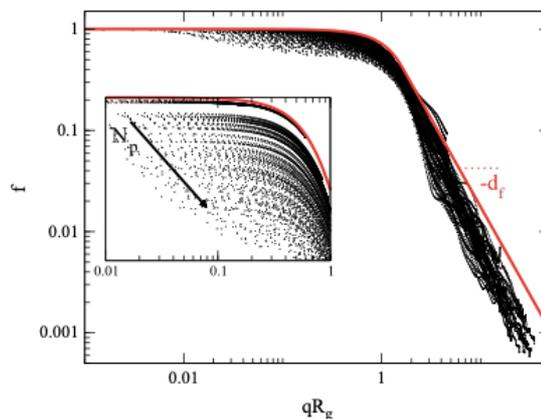
Figure 1: Comparison between rigorous calculations (DDSCAT, black dots) of aggregate structure factor  $f$  and prediction by RDG-FA theory (solid red lines) at  $\lambda=266$  nm.
