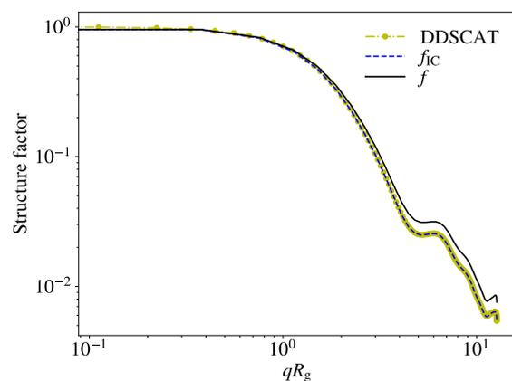
Figure 2: Comparison between DDSCAT calculation (circle marker) of aggregate structure factor and Eqs. (1) (solid line) and (3) (dashed line) for  $m = 1.1 + i0.8$
