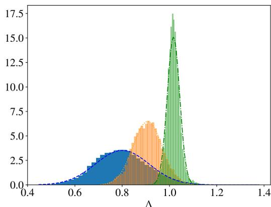
Figure 6: Probability density of the amplitude of the phasors for a fixed orientation of the aggregate for  $m=1.1+i0.01$  (in green dash dot line),  $m=1.1+i0.4$  (in orange dot line) and  $m=1.1+i0.8$  (in blue dashed line).
