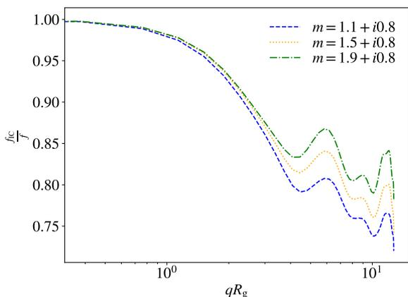
Figure 4: Deviation of  $f_{IC}$  with respect to  $f$  for  $m=1.9+i0.8$  (in green dash dot line),  $m=1.5+i0.8$  (in orange dot line) and  $m=1.1+i0.8$  (in blue dashed line).
