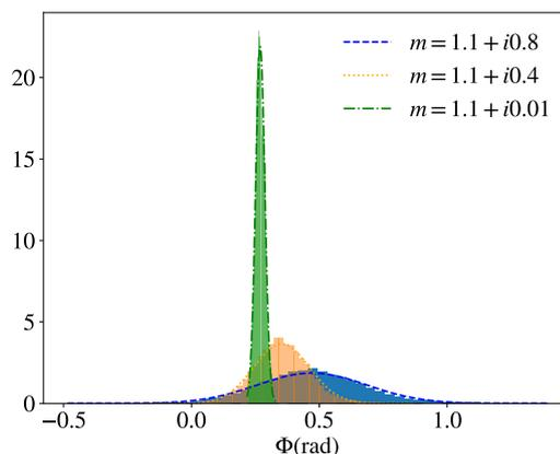
Figure 5: Probability density of the phase of the phasors for a fixed orientation of the aggregate for  $m=1.1+i0.01$  (in green dash dot line),  $m=1.1+i0.4$  (in orange dot line) and  $m=1.1+i0.8$  (in blue dashed line).
