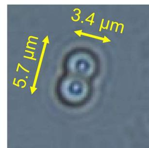
Figure 2 Microscope image of a hybrid silica "dumbbell" particle.
