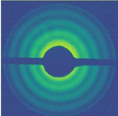
**Figure 3** Measured forward scatter image of a single hybrid silica sphere (presumably  $3.4\mu\text{m}$  diameter) in water at  $406\text{nm}$  wavelength. Logarithmic intensity scale.
