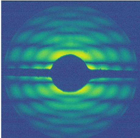
**Figure 5** Measured forward scatter image of a single hybrid silica dumbbell (3.4 $\mu\text{m}$  wide, 5.7 $\mu\text{m}$  long).
