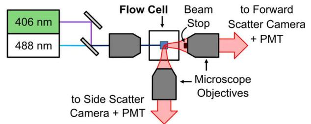
Figure 1 Cytometer flow cell with lasers and objectives. The flow direction is into the image plane.
