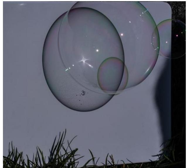
Figure 2 Glare points on the surface of a spheroidal floating bubble, and a cross section through the near-zone sagittal astroid caustic on a viewing screen behind the bubble.
