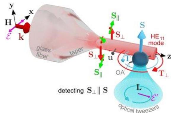
**Figure 1** Schematic of the experiment for a demonstration of the transverse spin of light. An anisotropic particle is trapped using an optical tweezers and placed in the evanescent field of an optical nanofibre. An optical torque  $T_{\perp}$  is produced via the transverse spin of light  $S_{\perp}$  and this contributes to the total torque  $T$  on the particle [9].
