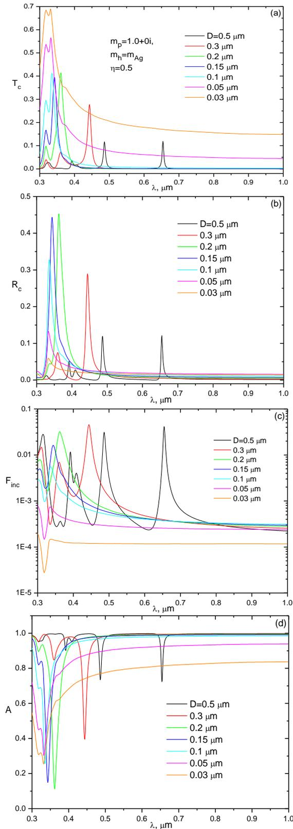
**Figure 2** Spectral dependences of  $T_c$ ,  $R_c$ ,  $F_{\text{inc}}$  and  $A$  coefficients of the partially ordered monolayer of spherical voids in silver (Ag) plate at different diameters  $D$  of voids.  $\eta=0.5$
