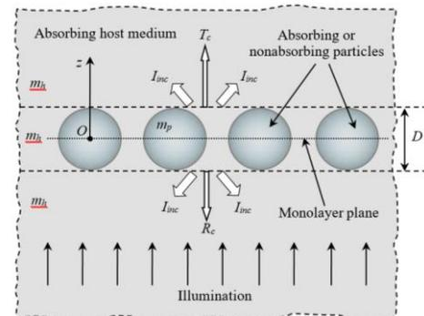
**Figure 1** Schematic view (along the monolayer plane) of normally illuminated monolayer of spherical particles embedded in absorbing host medium (matrix).  $T_c$  and  $R_c$  are coherent transmission and reflection coefficients of the system consisting of the monolayer of particles with diameter  $D$  and matrix layer with thickness  $D$ .  $I_{inc}$  is the intensity of the incoherent light.
