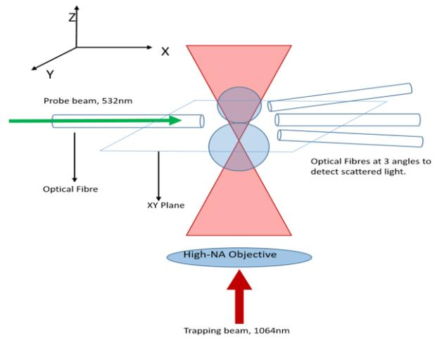
*Figure 1: Schematic of Light scattering detection from an optically trapped asymmetric microsphere doublet. The optical fibre carrying the probe beam and the 3 fibres used to detect scattered light are all in the XY plane. The reference frame is assumed to be coincident with the trap-centre and the z-axis is assumed to be along the propagation direction of the trapping beam*
