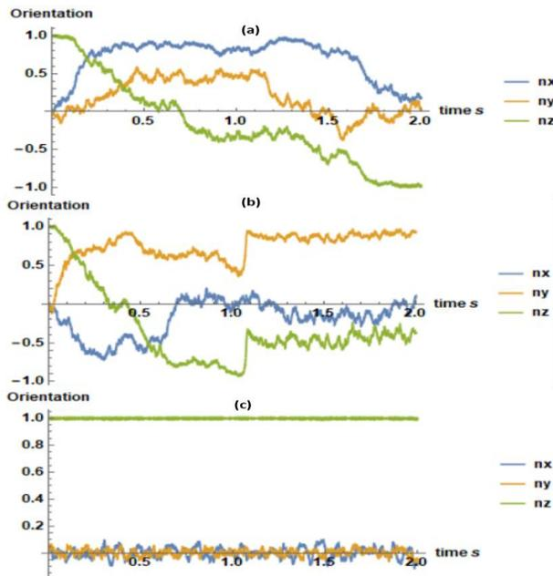
**Figure 2** Time evolution of orientation of dimers of radii (a)1:0.5-micron (b) 1:0.2-micron and (c) 1:1-micron. Dimers are suspended in water at 25°C and are being trapped in an Optical Trap of NA 1.2.
