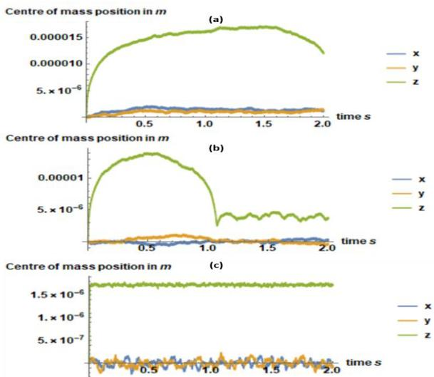
**Figure 3** Time evolution of the position of the centre of mass of dimers of radii (a)1:0.5-micron (b) 1:0.2-micron and (c) 1:1-micron. These positions are being reported with respect to the centre of the laser-trap
