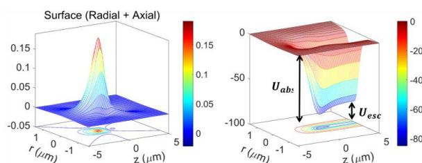
**Figure 2** Force (left panel) and potential (right panel) on an 80 nm diameter polystyrene bead under femtosecond pulsed excitation at 100 mW time-averaged power.
