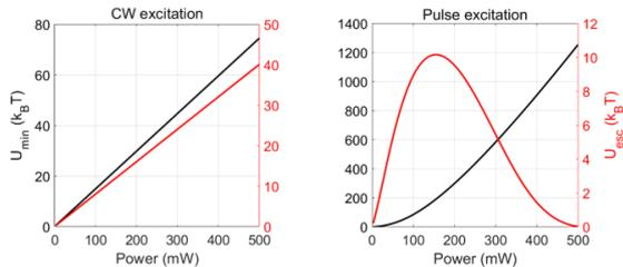
**Figure 3** Variation of absolute potential (black curves) and escape potential (red curves) with increasing time-averaged power for CW excitation (left panel) and femtosecond pulsed excitation.
