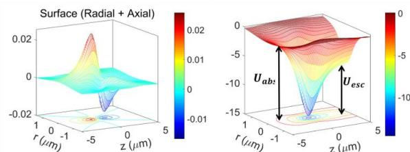
**Figure 1** Force (left panel) and potential (right panel) on an 80 nm diameter polystyrene bead under CW excitation at 100 mW time-averaged power.
