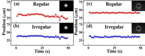
**Figure 2** The stability of regular and irregular particles using the vertical optical trapping scheme. (a) The regular particle in Gaussian trap; (b) The irregular particle in Gaussian trap; (c) The regular particle in hollow beam trap; and (d) The irregular particle in hollow beam trap.
