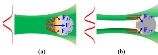
**Figure 6** The force analysis of particle in Gaussian and hollow traps.
