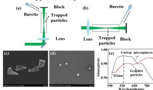
**Figure 1** (a) Scheme of the vertical trapping configuration; (b) Scheme of the horizontal trapping configuration; (c) The SEM image of the irregular graphite; (d) The SEM image of the carbon microspheres; (e) The infrared absorption spectra of the graphite particles and carbon microspheres.
