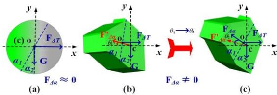
**Figure 5** The force analysis of the horizontal optical trapping schemes. The direction of laser is from left to right. (a) is the force analysis of regular particle; (b) is the force analysis of irregular particle.
