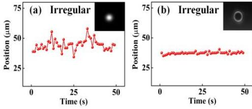
**Figure 3** The stability of irregular particles using the horizontal optical trapping scheme. (a) Gaussian beam trap (b) Hollow beam trap.
