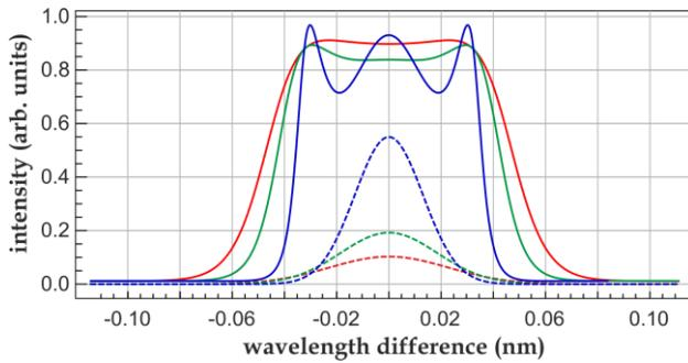
**Figure 2** Simulated spectra of the Thomson and Rayleigh scattering of 532 nm laser beam on the hydrogen plasma under the pressure 1000 mbar. Simulations were made for parameters:  $N_e = 0.3 \times 10^{23} \text{ m}^{-3}$ ,  $T_e = 13000 \text{ K}$ , and for the ratio  $T_e/T_i$  equal to 4/3 (red line), 2 (green line) and 4 (blue line). The Rayleigh scattering spectrum is marked with a dashed line. The sum of Rayleigh and Thomson scattering spectra is marked with a solid line.
