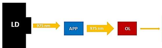
**Figure 1** Self-made optical system for up-conversion luminescence based lithographic recording
